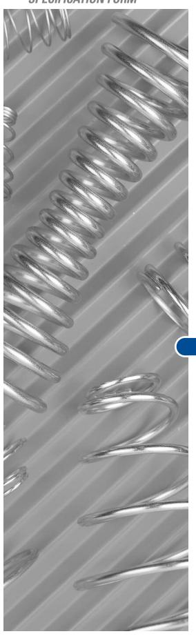
Coned compression springs are often specified when the large end is meant to work in a hole and the small end is meant to work over a rod. They offer the advantage of a reduced solid height compared to straight compression springs particularly when designed to telescope.
